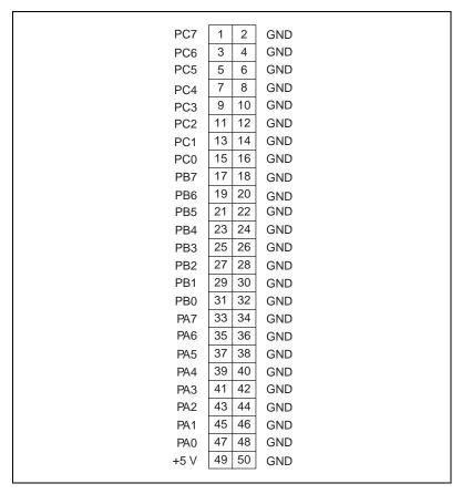
Figure B-5. 50-Pin DIO Connector Pin Assignments
