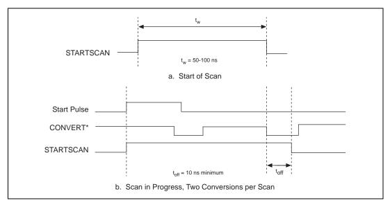
Figure 4-22. STARTSCAN Output Signal Timing
