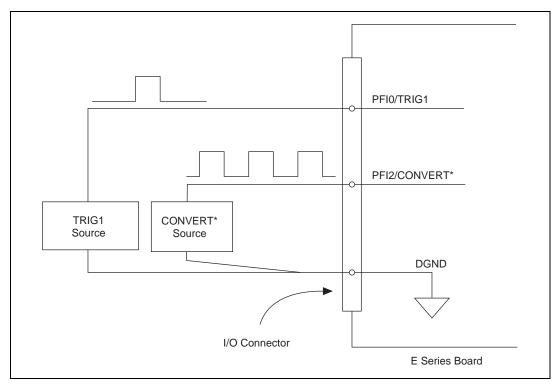
Figure 4-12. Timing I/O Connections
