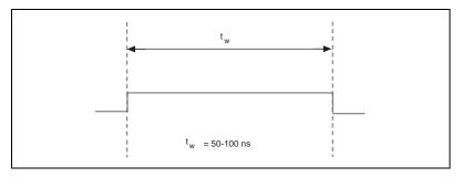
Figure 4-20. TRIG2 Output Signal Timing
