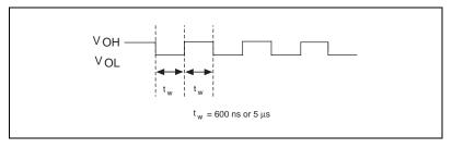
Figure 4-16. EXTSTROBE\* Signal Timing
