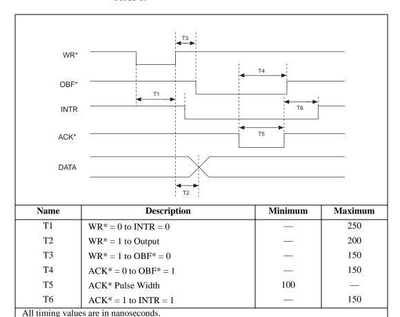
Figure 4-39. Mode 1 Output Timing
