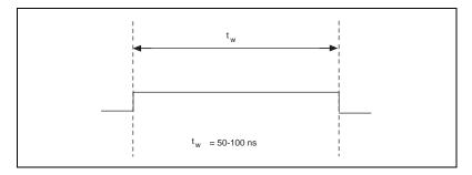
Figure 4-18. TRIG1 Output Signal Timing
