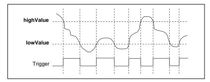
Figure 3-11. Inside-Region Analog Triggering Mode
