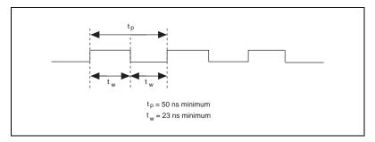
Figure 4-25. SISOURCE Signal Timing
