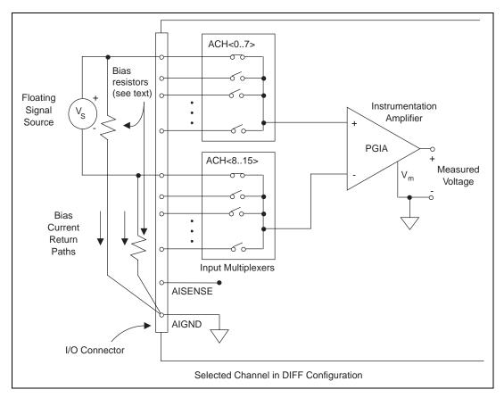
Figure 4-7. Differential Input Connections for Nonreferenced Signals
