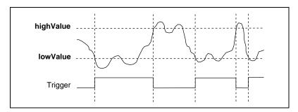
Figure 3-13. Low-Hysteresis Analog Triggering Mode
