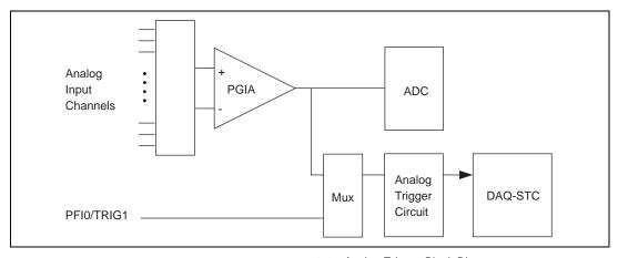
Figure 3-8. Analog Trigger Block Diagram
