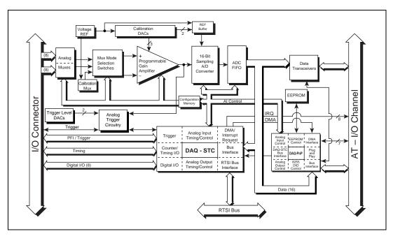
Figure 3-5 shows a block diagram for the AT-AI-16XE-10.
