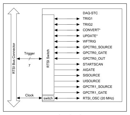
Figure 3-15. RTSI Bus Signal Connection
