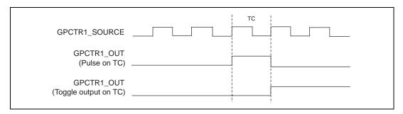
Figure 4-36. GPCTR1\_OUT Signal Timing
