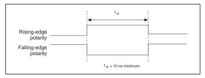
Figure 4-35. GPCTR1\_GATE Signal Timing in Edge-Detection Mode
