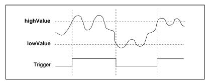
Figure 3-12. High-Hysteresis Analog Triggering Mode
