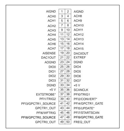
**Figure B-4.** 50-Pin MIO Connector Pin Assignments
