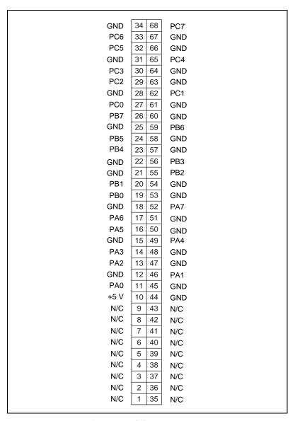
Figure B-2. 68-Pin DIO Connector Pin Assignments
