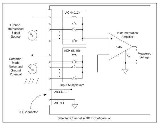
Figure 4-6. Differential Input Connections for Ground-Referenced Signals
