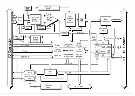
Figure 3-1. AT-MIO-16E-1 and AT-MIO-16E-2 Block Diagram
