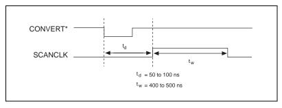
Figure 4-15. SCANCLK Signal Timing
