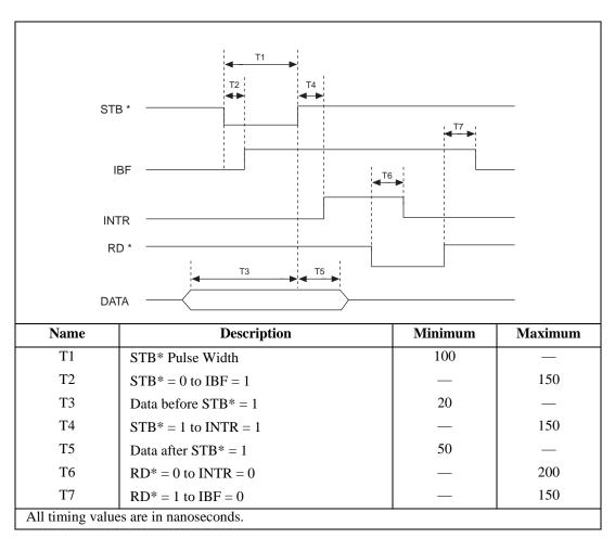
Figure 4-38. Mode 1 Input Timing
