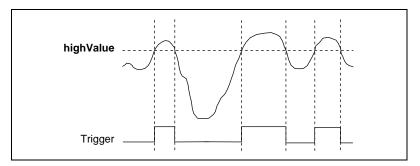
Figure 3-10. Above-High-Level Analog Triggering Mode
