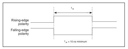
Figure 4-26. WFTRIG Input Signal Timing
