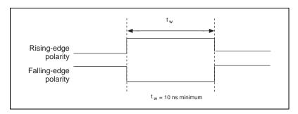
Figure 4-21. STARTSCAN Input Signal Timing
