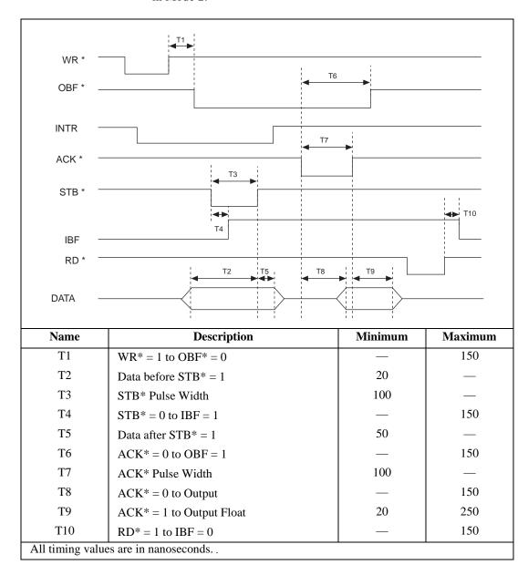
Figure 4-40. Mode 2 Bidirectional Timing
