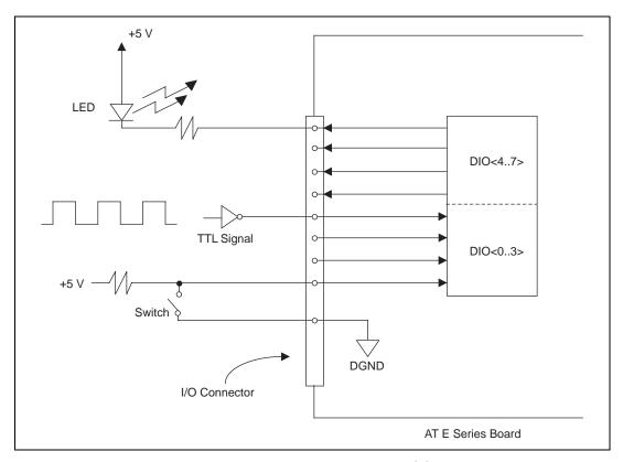
Figure 4-11. Digital I/O Connections
