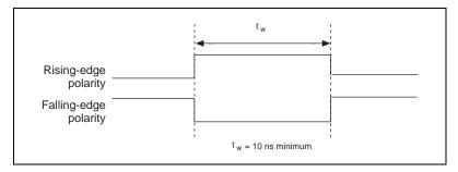
Figure 4-23. CONVERT\* Input Signal Timing
