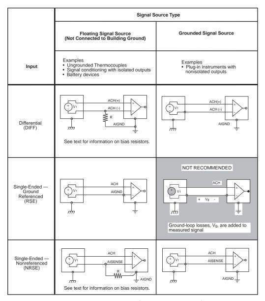
Figure 4-5. Summary of Analog Input Connections
