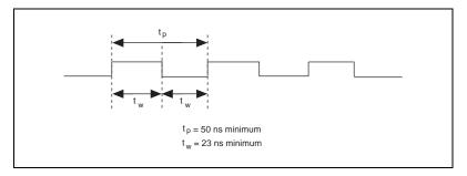
Figure 4-31. GPCTR0\_SOURCE Signal Timing
