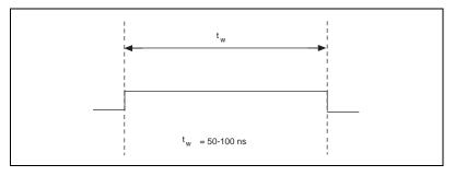
Figure 4-27. WFTRIG Output Signal Timing
