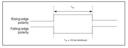
Figure 4-19. TRIG2 Input Signal Timing
