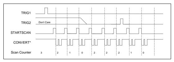
Figure 4-14. Typical Pretriggered Acquisition
