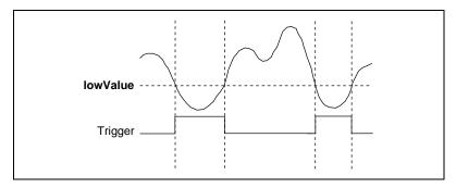
Figure 3-9. Below-Low-Level Analog Triggering Mode
