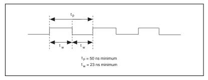
Figure 4-30. UISOURCE Signal Timing
