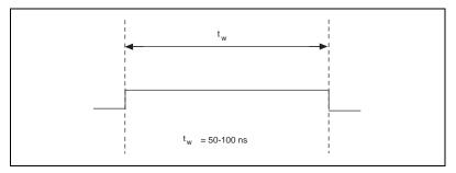
Figure 4-24. CONVERT\* Output Signal Timing
