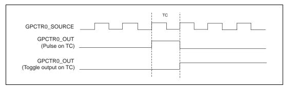
Figure 4-33. GPCTR0\_OUT Signal Timing
