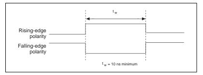
Figure 4-28. UPDATE\* Input Signal Timing
