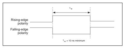
Figure 4-17. TRIG1 Input Signal Timing
