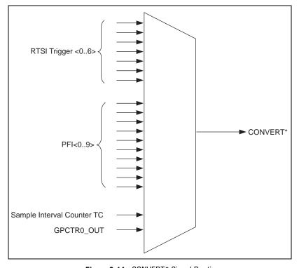
Figure 3-14. CONVERT\* Signal Routing
