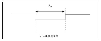
Figure 4-29. UPDATE\* Output Signal Timing
