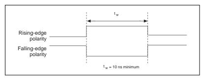
Figure 4-32. GPCTR0\_GATE Signal Timing in Edge-Detection Mode
