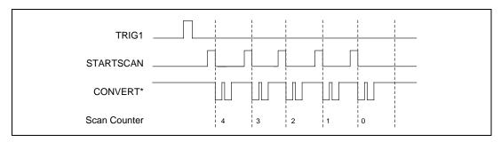
Figure 4-13. Typical Posttriggered Acquisition
