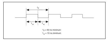
Figure 4-34. GPCTR1 SOURCE Signal Timing
